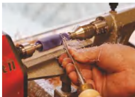
▲ Pic.5 Turn the acrylic on a fast speed for best results, keeping the chisel angles to shear the cut
